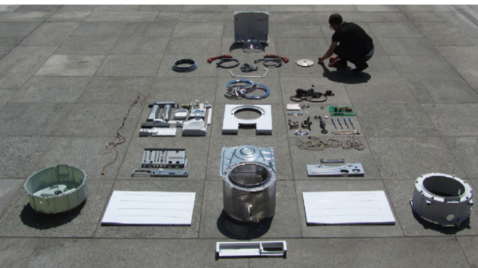
A dismantled Adora washing machine lays the foundations for a life cycle assessment
